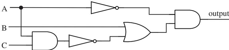
Figure 2.3: The standard symbols for the three basic logic gates, and a logic circuit that computes the value of the logical expression  $(\neg A) \wedge (B \vee \neg(A \wedge C))$ . The input wires to each logic gate are on the left, with the output wire on the right. Note that when wires cross each other in a diagram such as this, the wires don't actually intersect unless there is a black circle at the point where they cross.
