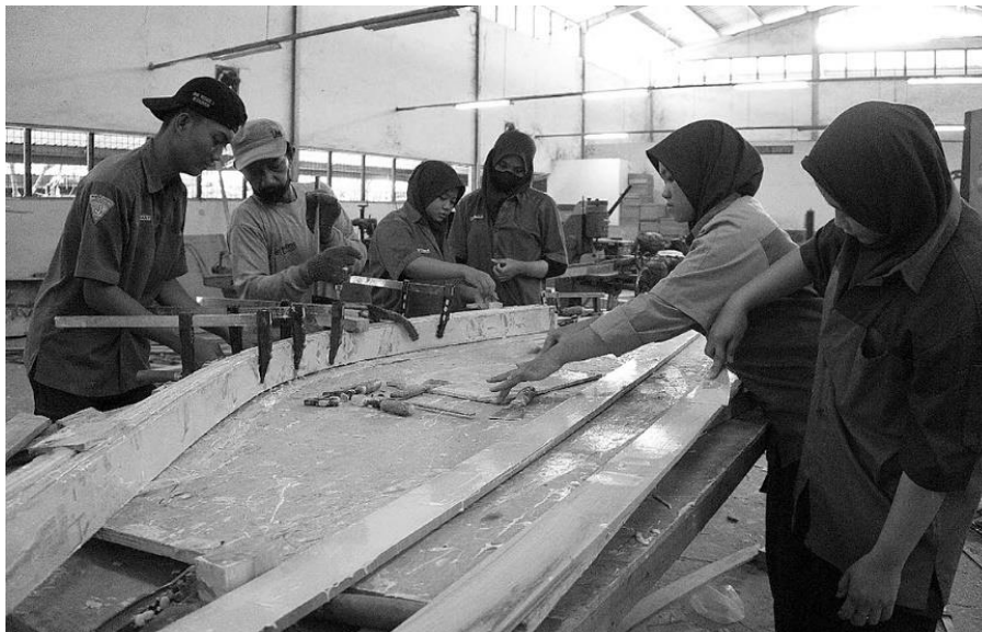
Figure 4: The students are constructing the boat's laminated frames in the school workshop
