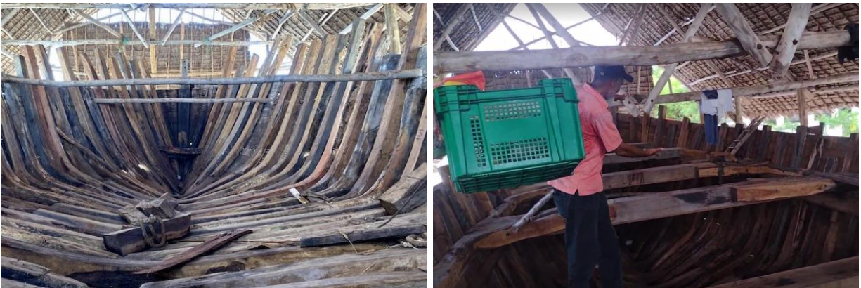
Figure 13: The original ribs of Utamaduni in the Flipflop boatyard (left) and the renewed structure (right)
