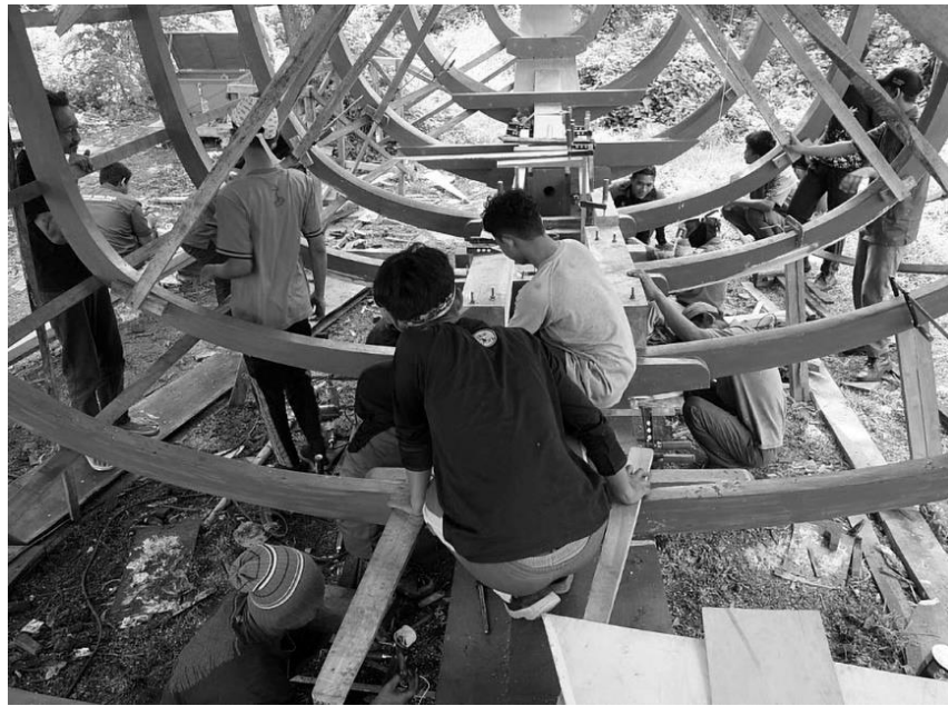
Figure 5: The students are working on setting the frames in the boatyard.
