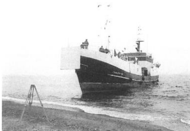
Figure 11: Full Ship Grounding Experiments Conducted by Sterndorff & Pederson (1996)
