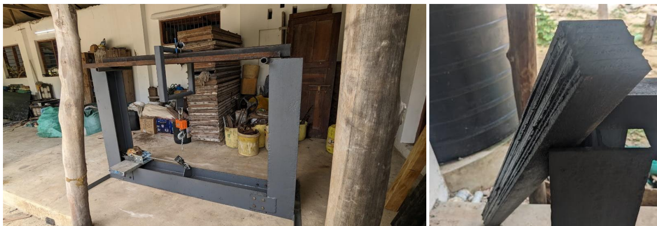
Figure 23: The 3-point structural test rig (left), a 4” x 4” HDPE laminated beam (right)
