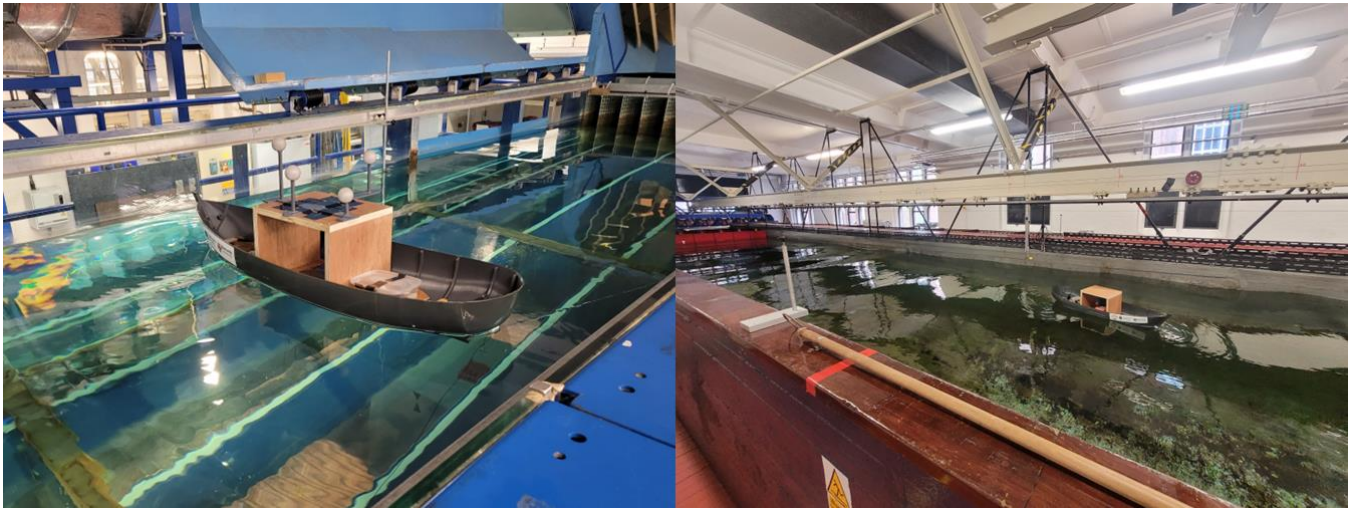
Figure 4: Model in Testing Facilities, Newcastle University. Wind Wave Current Tank (left), Towing Tank (right)
